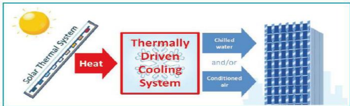
Figure 7: Simplified illustration of a solar cooling system, which can provide cooling by chilled water or by delivering conditioned air.(URL 4)
